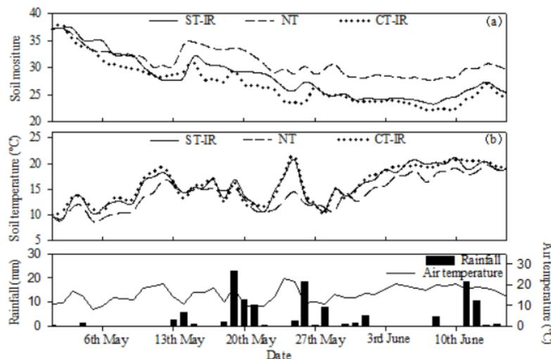
**Figure 3.** Dynamic changes of soil moisture (a) and soil temperature (b) under different tillage treatments at the depth of 0–10 cm in 2019.
