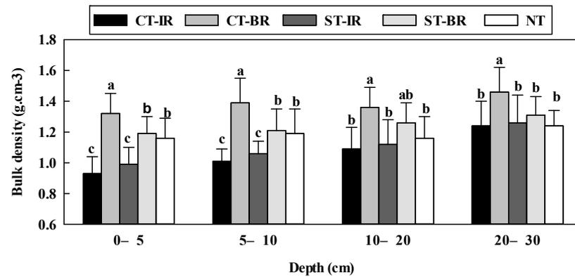
**Figure 1.** Differences in bulk density among the different tillage treatments. Notes: Values followed by the different lowercase letters in the same depth had significant differences at 0.05 level. ST: Strip tillage; NT: no tillage; CT: conventional tillage; IR: within the tilled planting row; BR: between the planting rows.
