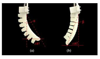
Figure 7. Experimental results: (a) inflation status; (b) deflation state.
