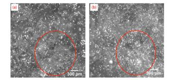
**Figure 14.** Apple surface under 5 times microscope. (**a**) apple held by flexible gripper. (**b**) apple held by rigid gripper.
