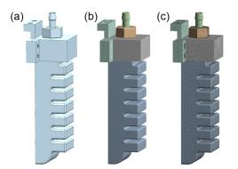
Figure 5. Model flexible finger: (a) UG model; (b) ANSYS model; (c) grid chart.
