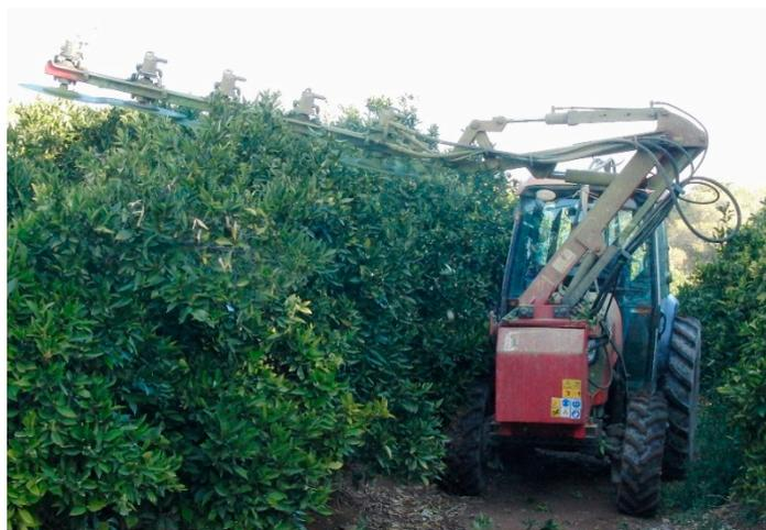
**Figure 1.** The tractor disc pruner used in the trials.
