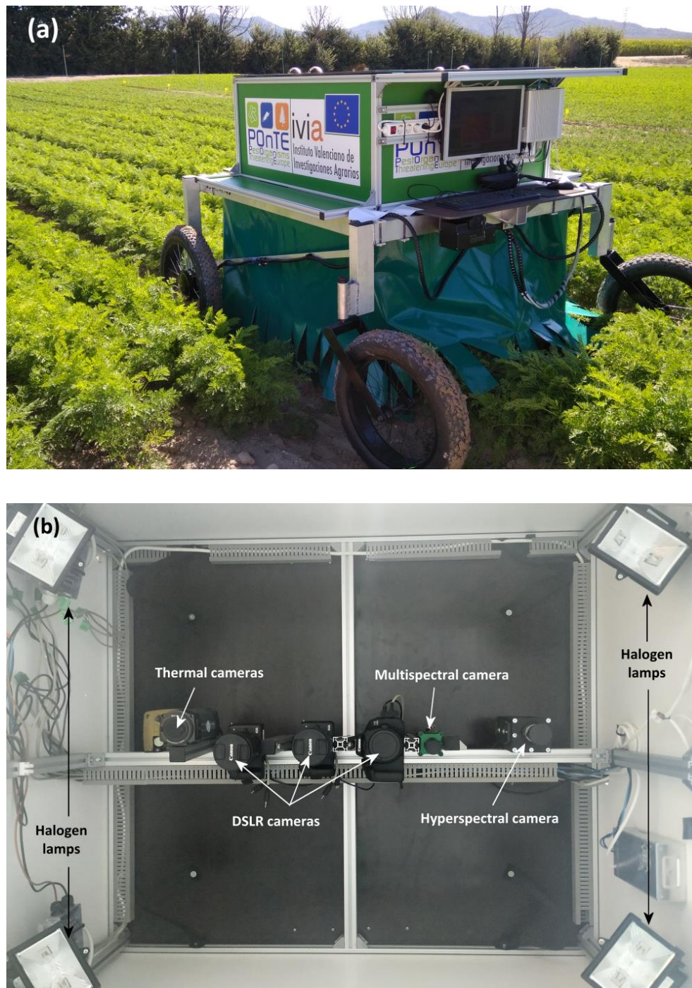
Figure 3. A remotely-driven RobHortic operating in a carrot field. (a) the external appearance of the robot. (b): inside from the plant point of view.
