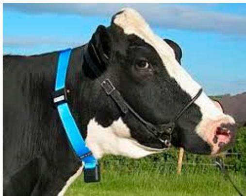
**Figure 1.** Silent Herdsman (Afimilk Ltd., Kibbutz, Afikim, Israel) 3-axis accelerometer based neck-mounted collar.
