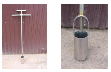
Figure 1. Soil sampling tube.
