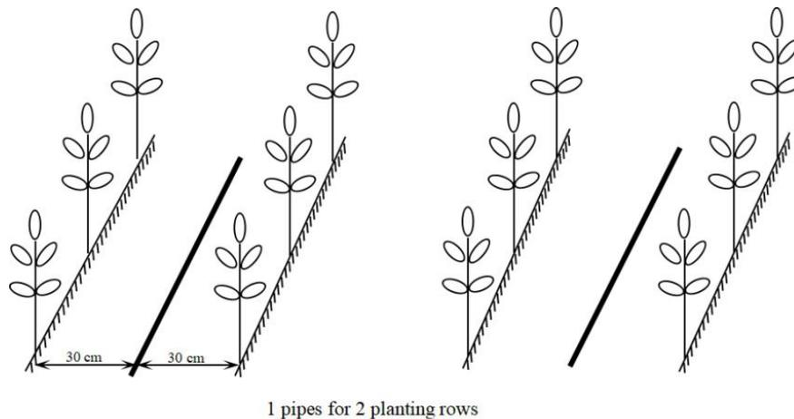
**Figure 1.** Diagram of drip irrigation pipe density.
