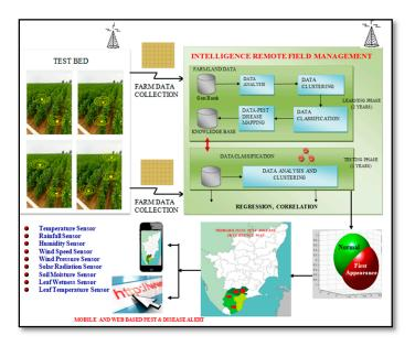
Figure 1. System architecture of the intelligent pest and disease forewarning model.
