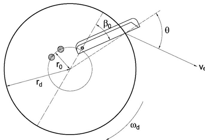
**Figure 2.** Geometry, kinematics, and dynamics of a spinning disc fertilizer.
