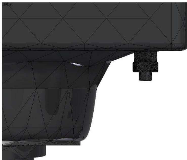
Figure 14. Detail of automatic meshing in elements of complex geometry.
