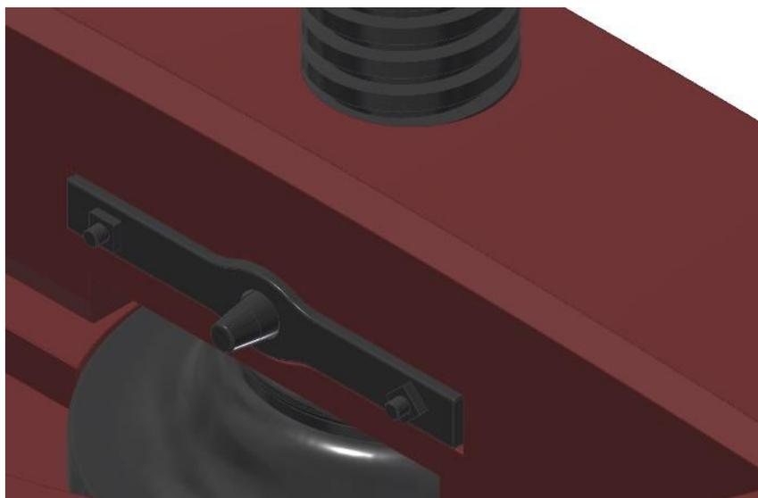
Figure 16. Screw attached to the nut by means of a frusto-conical bolt with some looseness.
