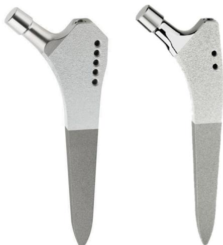
**Figure 1.** The SL-PLUS stem on the left side and the SL-PLUS MIA stem on the right side. Both stem designs are based on the Zweymüller concept with a proximal hydroxyapatite coating in order to facilitate bone ingrowth. For the SL-PLUS MIA stem the metaphyseal geometry was modified with a less prominent lateral shoulder in order to facilitate a bone preserving implantation.
