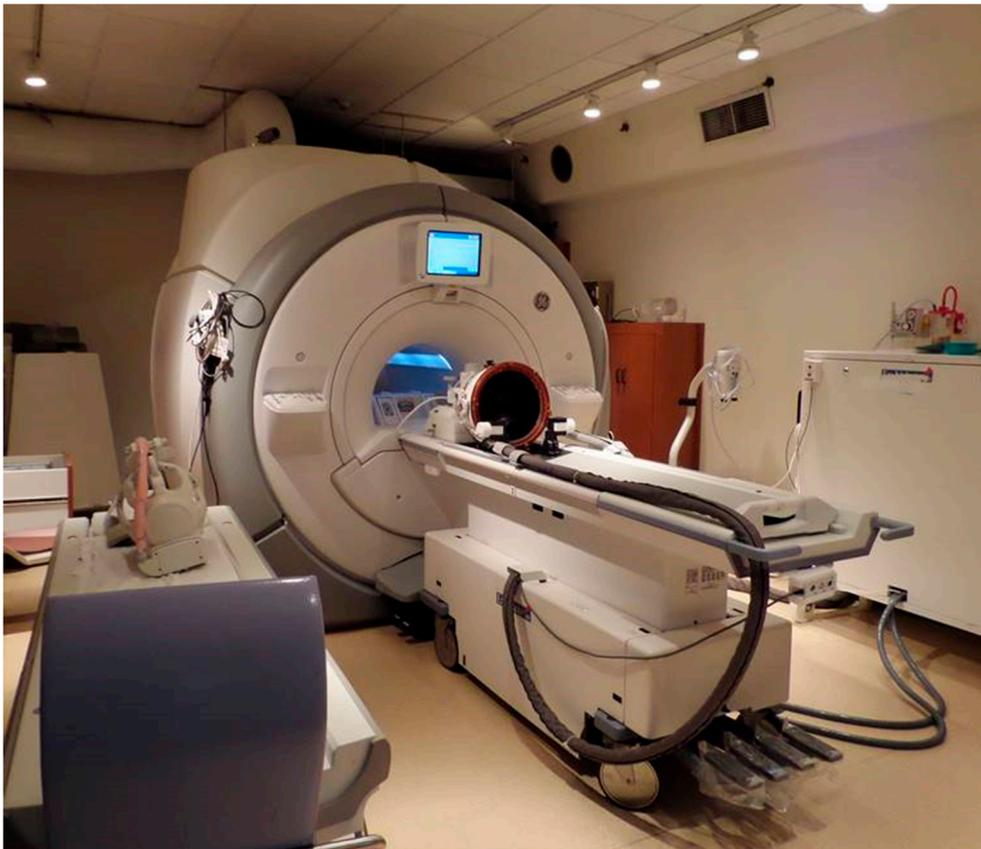
**Figure 5.** An ExAblate Neuro (InSightec, Haifa, Israel) MRgFUS transducer helmet on an MRI table (located at Sunnybrook hospital, Toronto, Canada).
