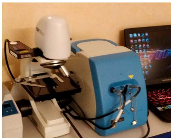
**Figure 1.** The Raman setup used in this study. The picture shows the portable Raman spectrometer coupled with a microscope.
