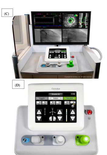
**Figure 1.** The CorPath GRX system. The robotic arm and disposable cassette is shown in (**A**). The arm extends freely from the table mount to allow variable configurations for catheter attachment (**B**). The interventional cockpit is shown in (**C**) with a close up of the workstation showing the joystick controls in (**D**). (Provided by and with permission from Corindus Vascular Robotics, Boston, MA, USA).
