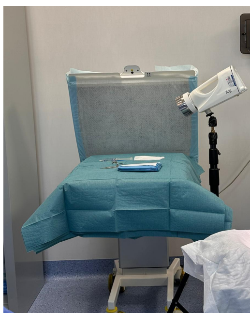
Figure 2. The SAS device is positioned within the laminar airflow for air sampling. The photo shows the filter drape protecting the instrument area under laminar airflow.
