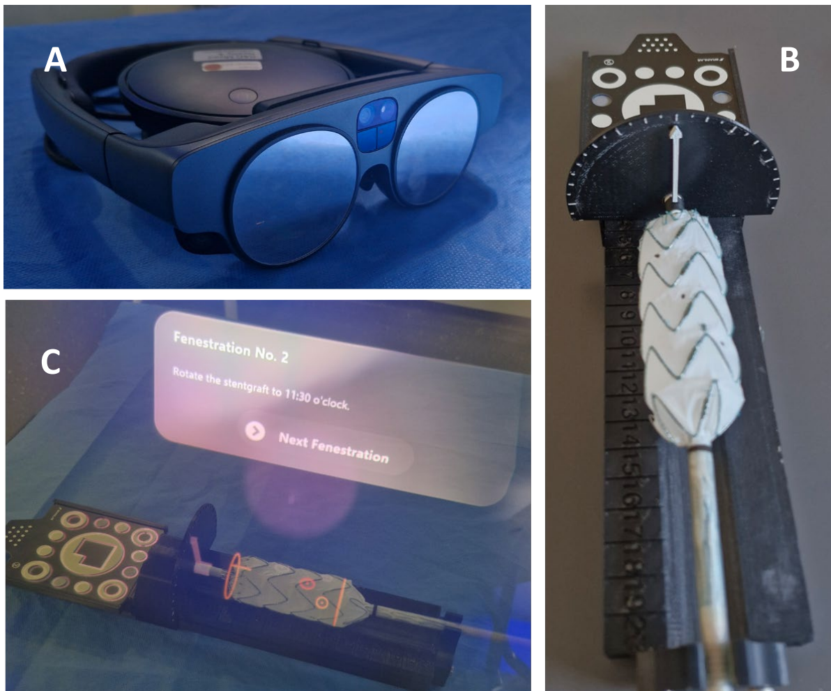
Figure 1. (A) Magic Leap 2 (Plantation, USA) head-mounted display; (B) template device; and (C) operator's point of view performing MxR-assisted PMEG.
