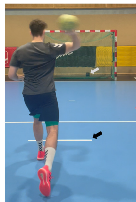
Figure 1. Handball throwing velocity testing setup. A player performing an overhead throw from behind the 7 m free-throw line (black arrow). The radar gun (gray arrow) was positioned behind the net to record the throwing velocity.
