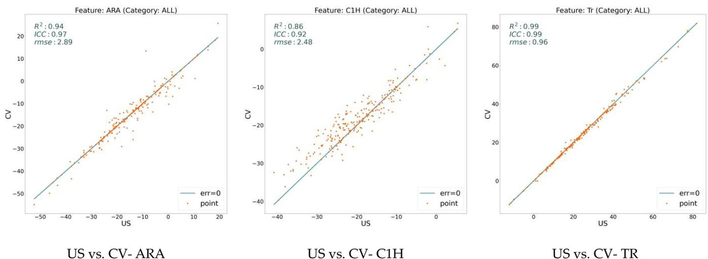
**Figure 2.** Error analysis between human expert (US) and the model (CV) over three general features, including ARA, C1H, and TR. While x-axis shows the feature value calculated based on the expert's annotation, y-axis determines the value based on the model's prediction. The points on the line have zero errors.
