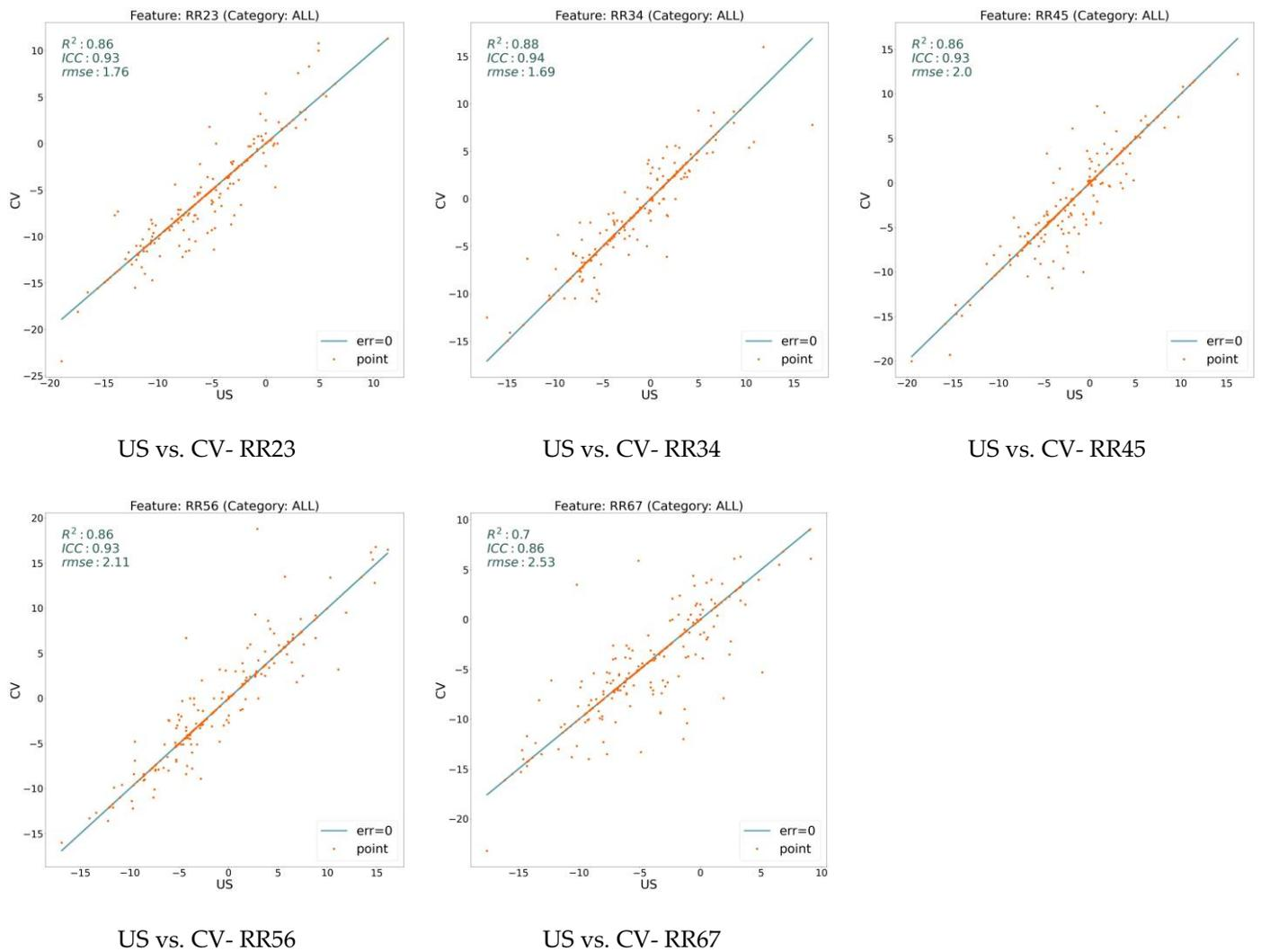
**Figure 4.** Error analysis between human expert (US) and the model (CV) over RRA (RR) feature. While x-axis shows the feature value calculated based on the expert’s annotation, y-axis determines the value based on the model’s prediction. The points on the line have zero errors.
