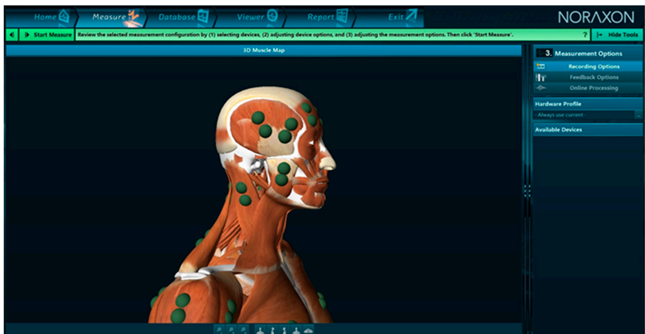
Figure 4. Graphic showing the position of the temporalis and masseter muscle electrodes according to the SENIAM program. Screen from Noraxon MR3 3.18.08 software (Noraxon USA, Inc., Scottsdale, AZ, USA).
