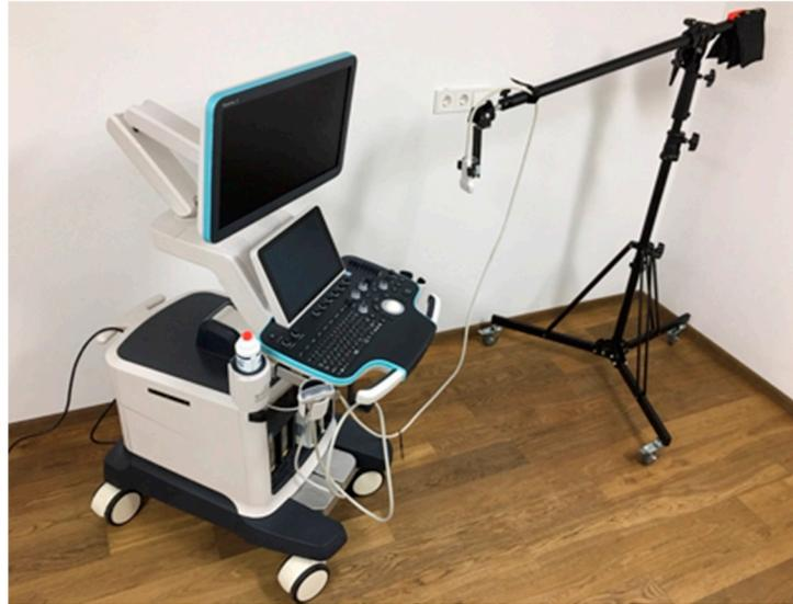
**Figure 6.** Ultrasound probe with fixation arm.
