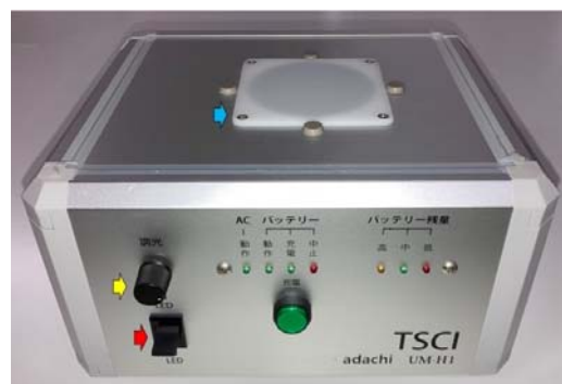
Figure 1. Main unit of TSCI. On the front of the device, there is a tab to switch the 605 nm wavelength light (red arrow), a knob to adjust the light intensity (yellow arrow), and a lamp to check the operation status. In the center of the upper surface of the device, there is a white plate that emits transmitted light from below, and a Petri dish containing the specimen is placed on this plate (blue arrow). Abbreviation: TSCI, target sample check illuminator.
