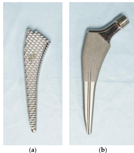
Figure 1. Anterior views of (a) broach and (b) stem with single-wedge design. The stem is 0.25 mm smaller on both the medial and lateral sides than the broach, but the coating on the distal 10 mm length of the sprayed area increases in a gradient from distal (0.2 mm) to proximal (0.5 mm). The stem and broach were manufactured by Kyocera Corporation (Kyoto, Japan).
