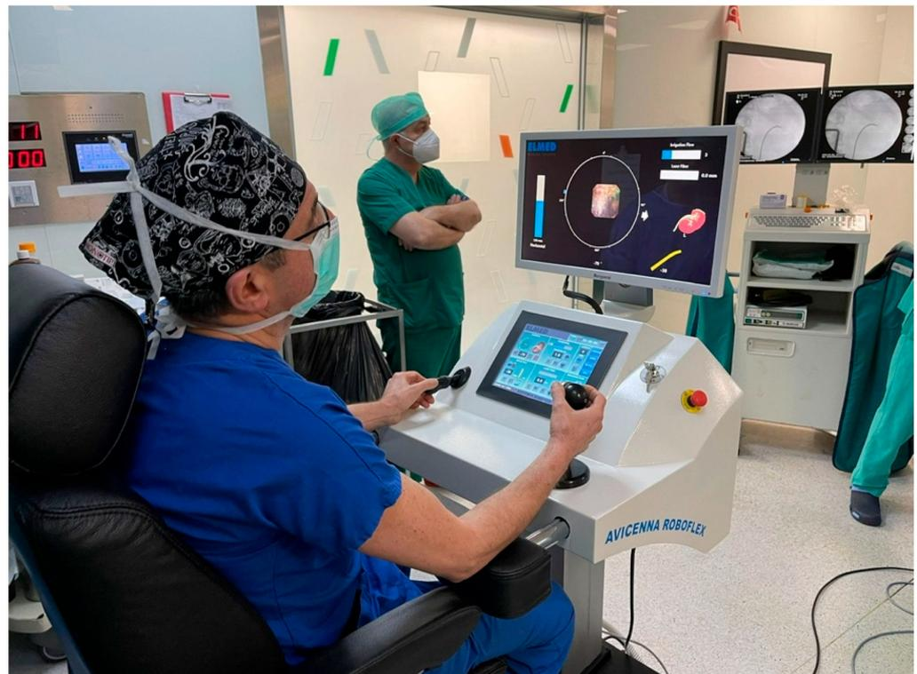
**Figure 2.** Surgeon working at the Roboflex Avicenna console.
