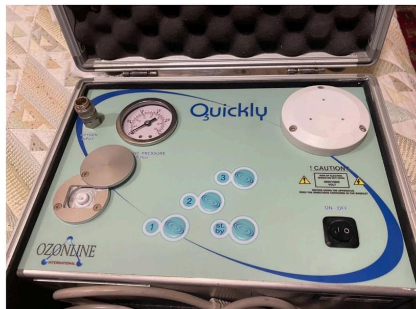
**Figure 1.** Device for the generation of ozone by transformation of medical oxygen (the Quickly by Ozonline<sup>®</sup> (ECO3, Sevilla, Spain)).
