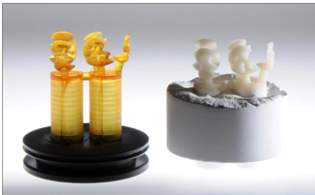
Figure 17. Comparison of 3D printed and pressed ceramic inlays.
