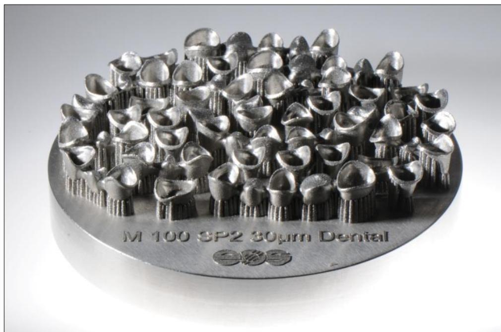
**Figure 3.** Lasersintered CoCr Crowns and Bridges.
