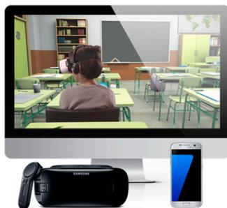
**Figure 2.** Aula Nesplora (virtual reality continuous performance test) hardware.
