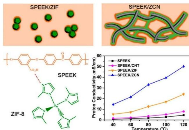
**Figure 19.** Interaction between SPEEK and ZIF-8, and the schematic illustration for the interface of SPEEK/ZIF and SPEEK/ZCN composite membranes. Reprinted with permission from Ref. [59]. Copyright 2017 American Chemical Society.
