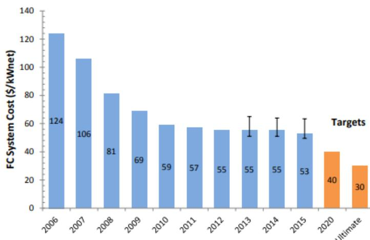
**Figure 1.** Cost-analysis of an 80 kW<sub>net</sub> automotive PEMFC-based on projection to a volume of 500,000 units/year [10].
