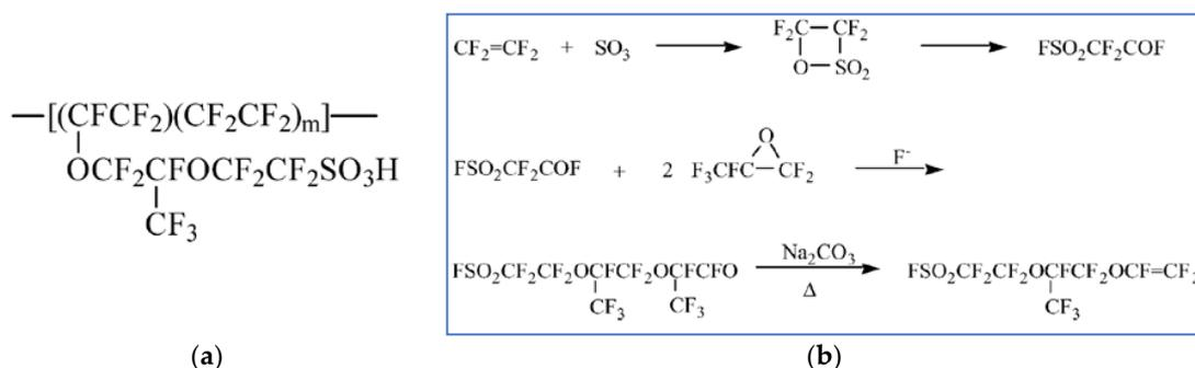
**Figure 3.** The chemical structure of Nafion (a) and the synthesis process for the vinyl ether monomers, the starting point for Nafion (b). (b) is reprinted with permission from Ref. [20]. Copyright 2004 Elsevier.
