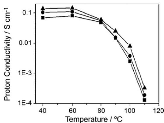
**Figure 8.** The proton conductivity of membranes without external humidification. Triangle is zirconia-doped, circle is silica-doped membrane and square is recast Nafion. Reprinted with permission from Ref. [48]. Copyright 2010 Elsevier.
