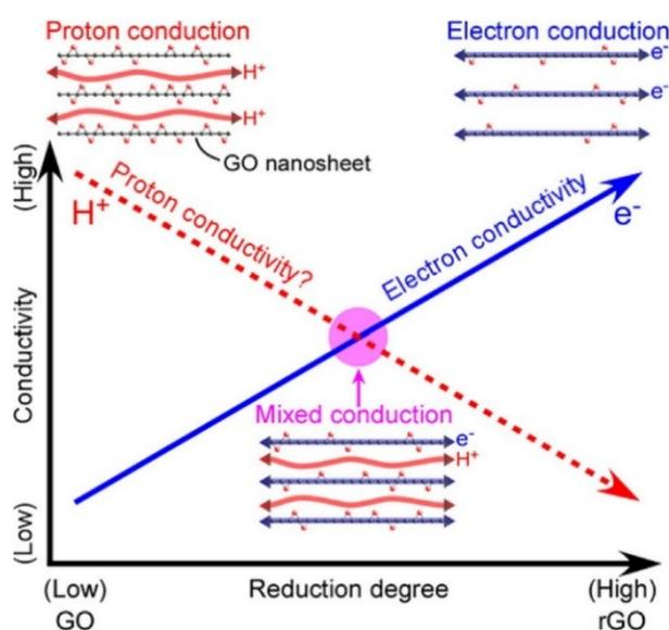
**Figure 24.** The concept behind the degree of GO reduction, which increases the electronic conductivity but decreases the protonic one. Reprinted with permission from Ref. [204]. Copyright 2014 American Chemical Society.
