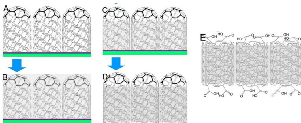
**Figure 23.** VANT membrane synthesis route. In green is the Si wafer, in blue an alumina support and in red an iron catalyst where the CNTs were grown (A); in grey the epoxy coating (B); tip exposure (C); removal of wafer and catalyst (D); tube opening via O<sub>3</sub> treatment (E). Reprinted with permission from Ref. [203]. Copyright 2014 American Chemical Society.
