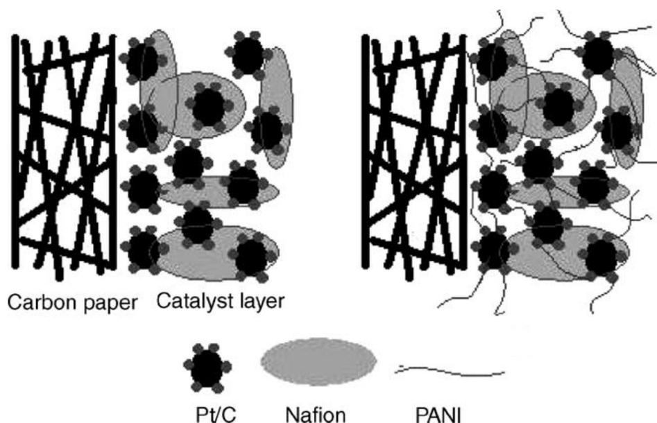
**Figure 22.** Schematic representation of the role of PANI nanofibers in connecting the catalyst particles embedded in the Nafion matrix. Reprinted with permission from Ref. [191]. Copyright 2006 Elsevier.
