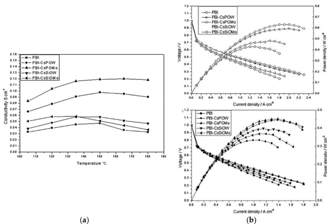
**Figure 14.** Proton conductivities of PBI composite membrane containing 30 wt.% CsHPA at ADL = 4.5, RH < 1% (a); polarization and power density curves of a PEMFC operated at 150 °C with H<sub>2</sub>/O<sub>2</sub> atmospheric pressure (upper plot) and H<sub>2</sub>/air atmospheric pressure (lower plot) (b). Reprinted with permission from Ref. [129]. Copyright 2011 Royal Society of Chemistry.
