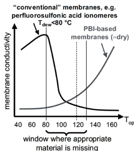
**Figure 5.** Membrane conductivity based on perfluorosulfonic acid (PFSA) ionomers and PBI, displaying the conductivity gap from 80 °C to 130 °C. Reprinted with permission from Ref. [28]. Copyright John Wiley & Sons, Ltd.
