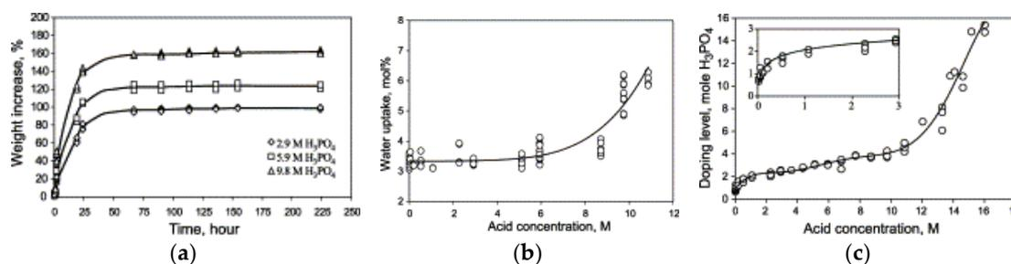
**Figure 11.** Weight increase as a function of time (a); water uptake (b); acid doping level of acid-doped PBI membranes at room temperature (c). Reprinted with permission from Ref. [100]. Copyright 2004 Elsevier.
