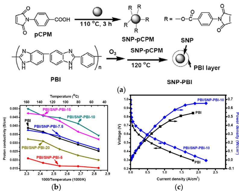
**Figure 12.** Ozone-mediated process for the synthesis of PBI/SNP-PBI nanocomposite membranes (a); proton conductivity of PBI/SNP-PBI membranes with different filler content (b); PEMFC polarization curve of PBI compared to PBI/SNP-PBI with 10 wt.%  $\text{SiO}_2$  membranes at  $150^\circ\text{C}$  using dry  $\text{H}_2/\text{O}_2$  as reactant at a flow rate of  $0.3 \text{ L/min}$  (c). Reprinted with permission from Ref. [112]. Copyright 2012 Elsevier.
