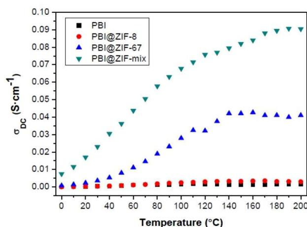
**Figure 17.** The temperature-dependent proton conductivity of  $H_3PO_4$ -doped PBI membrane and PBI composite membranes with 5 wt.% of ZIFs. Reprinted with permission from Ref. [57] under a Creative Commons Attribution (CC-BY) License. Copyright 2018 MDPI.
