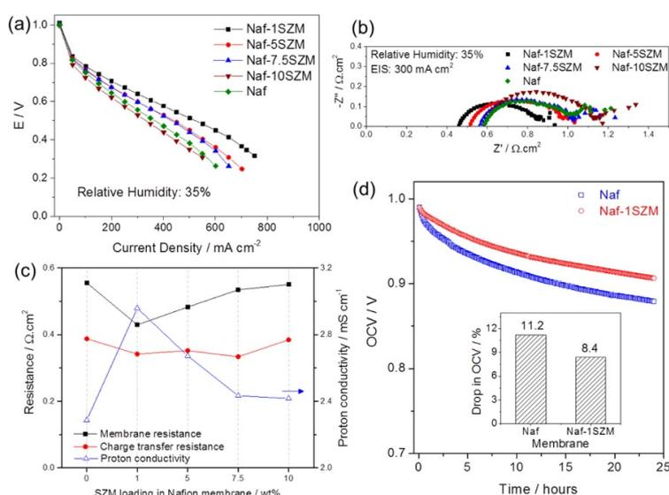
**Figure 10.** Polarization curves (a). Nyquist plots obtained with EIS (b), membrane resistances, proton conductivities and charge transfer resistances as a function of the SZM content in the composite (c). Stability runs as obtained for 24 h at 35% RH, at 80 °C (d). The inset shows the OCP drop in percentage (%). Reprinted with permission from Ref. [61] under a Creative Commons Attribution (CC-BY) License. Copyright 2016 American Chemical Society.
