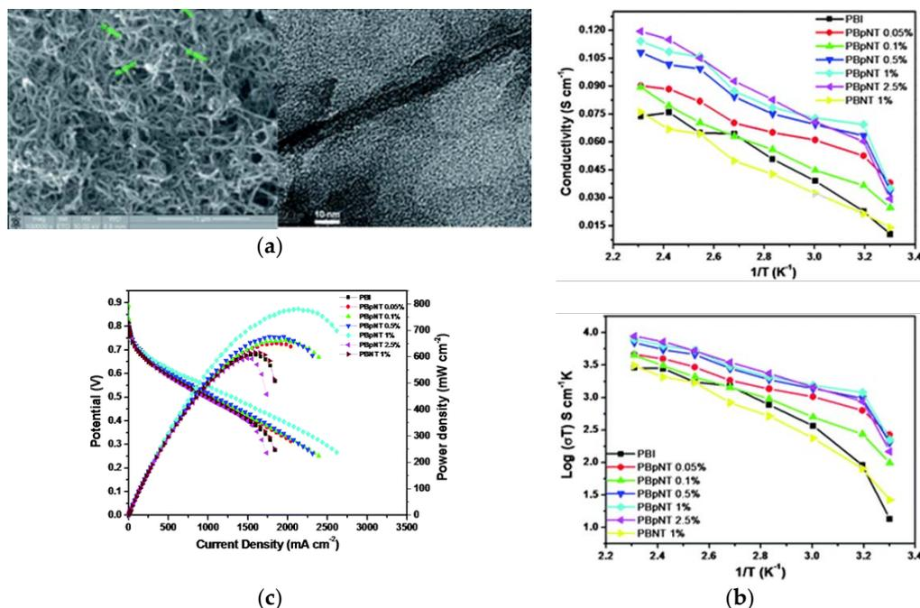
**Figure 15.** SEM image of p-MWCNTs and TEM image showing the distribution of p-MWCNTs inside the PBI matrix (a); proton conductivity and Arrhenius plots of the different composite membranes and pristine PBI (b); fuel cell polarization curves measured by supplying dry H<sub>2</sub>/O<sub>2</sub> with a flow rate of 0.2 standard liter per minute (slpm) at 140 °C (c). Reprinted with permission from Ref. [132]. Copyright 2011 Royal Society of Chemistry.
