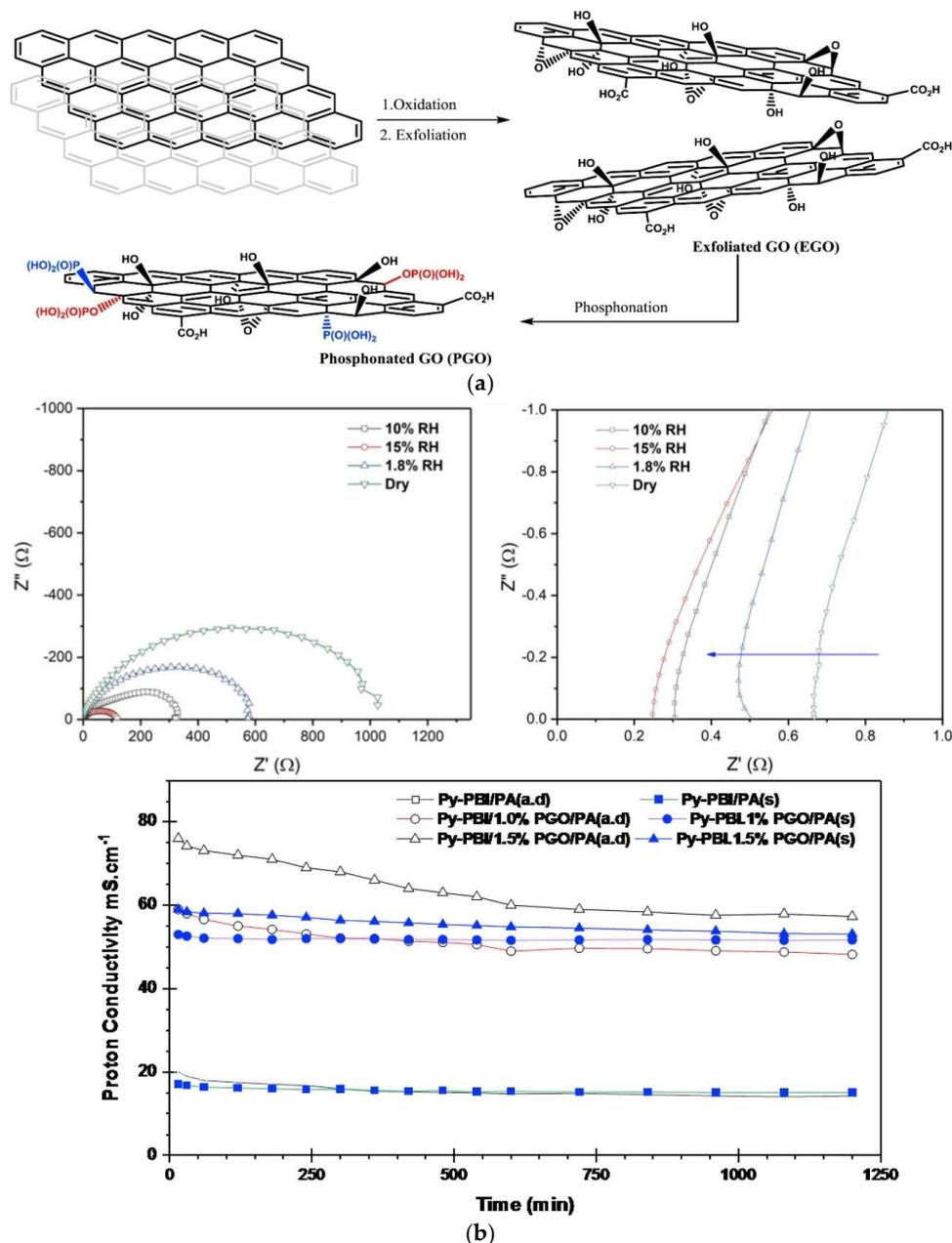
**Figure 16.** Preparation of functionalized graphene oxide (a); Nyquist plot of  $\text{H}_3\text{PO}_4$ -doped py-PBI/1.5 wt.% pGO under various RH at  $120 \text{ }^\circ\text{C}$ ; zoom-in in the high frequency intercept; and proton conductivity of the py-PBI composite membranes with different filler content as a function of testing time at  $140 \text{ }^\circ\text{C}$  and  $0\% \text{ RH}$  (b). Reprinted with permission from Ref. [136]. Copyright 2019 Elsevier.
