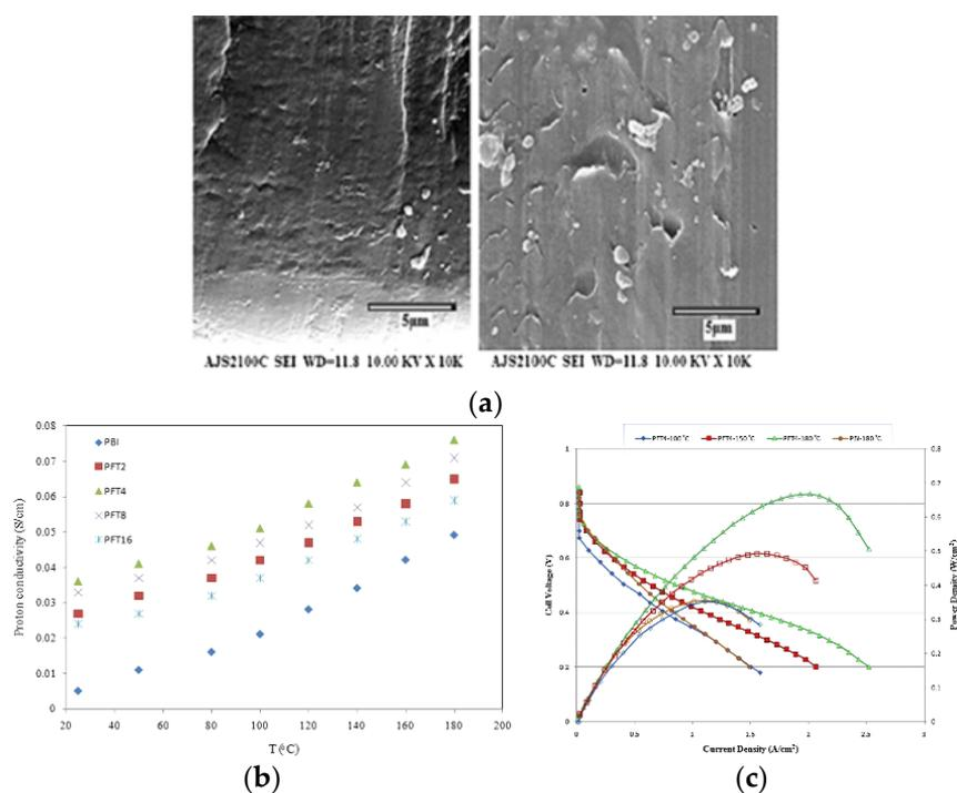
**Figure 13.** SEM cross-section image of  $\text{H}_3\text{PO}_4$ -doped PBI nanocomposite membrane with 4 wt.% and 16 wt.%  $\text{Fe}_2\text{TiO}_5$  nanoparticles (a); proton conductivity at RH = 0% (b); polarization curves for the single PEMFC of  $\text{H}_3\text{PO}_4$ -doped PBI with 4 wt.%  $\text{Fe}_2\text{TiO}_5$  nanocomposite membrane (c). Reprinted with permission from Ref. [108]. Copyright 2016 Elsevier.
