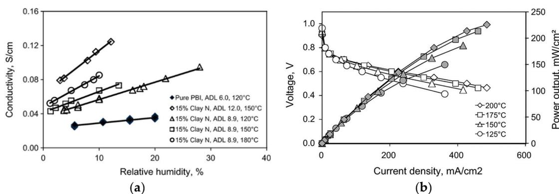
**Figure 18.** Conductivity of PBI membrane and PBI/clay N composites as a function of relative humidity at different temperatures (a); polarization curve for a fuel cell with PBI/5 wt.% clay L composite membranes (ADL = 8.2) obtained at different temperatures (b). Reprinted with permission from Ref. [141]. Copyright 2011 Elsevier.
