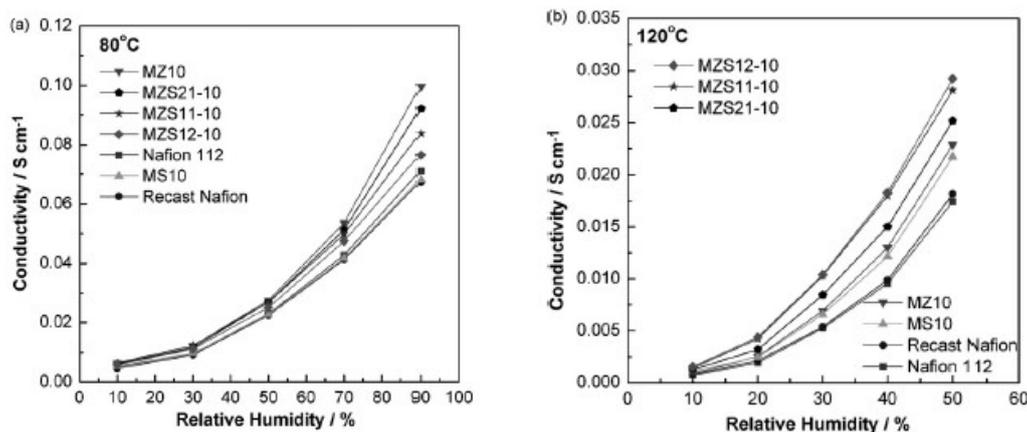
**Figure 9.** The measured conductivity of the membranes over different RH levels, where the membranes are labeled MZSxy-10 and x:y is Zr:Si, at 80 °C (a) and at 120 °C (b). Reprinted with permission from Ref. [49]. Copyright 2008 Elsevier.
