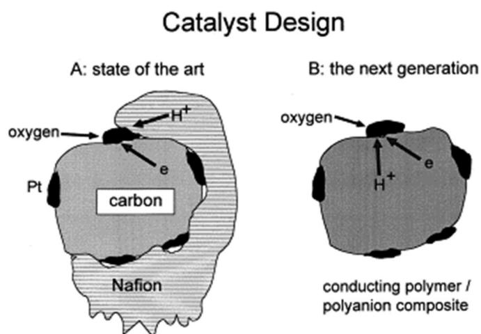
**Figure 21.** The commonly used electrode configuration (A) and the preferred design (B) in which the electronic conduction is added in parallel to the protonic one. Reprinted with permission from Ref. [166]. Copyright 1998 Elsevier.
