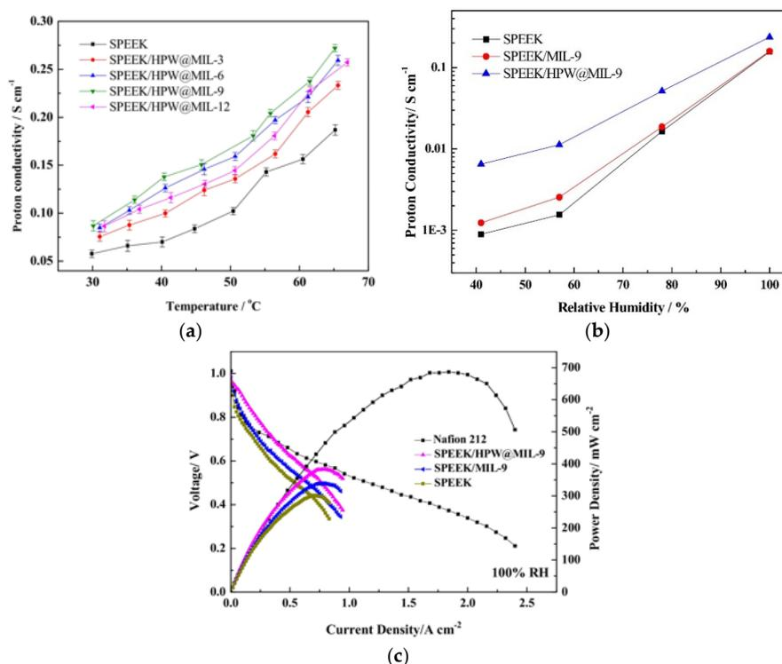
**Figure 20.** Proton conductivity of SPEEK/HPW@MIL101 membranes with different filler content at 100% RH under different temperatures (a); proton conductivity of the membranes with 9 wt.% HPW@MIL101 under different RHs (b); single H<sub>2</sub>/O<sub>2</sub> fuel cell performance (c). Reprinted with permissions from Ref. [63]. Copyright 2017 Elsevier.
