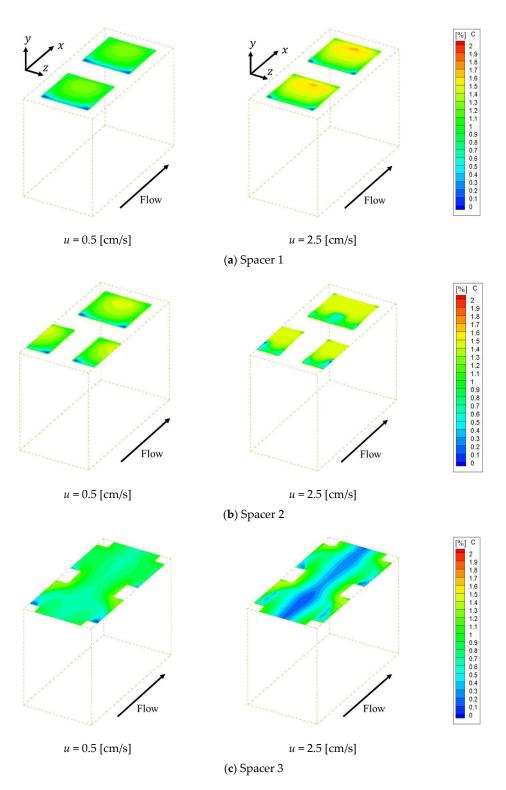
**Figure 4.** Concentration fields on an ion exchange membrane with porous spacers. (a,b) High concentration regions are formed at the attachment point of recirculation flow, while the low concentration regions are formed behind the structure; (c) Low concentration regions are observed on the center of the membrane along the main flow, which was not seen from (a,b).
