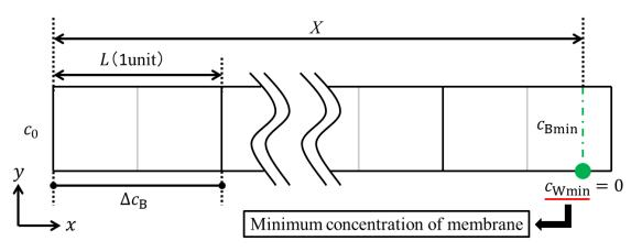
**Figure 2.** Limiting current density occurrence point. A point where water dissociation is occurring is located at the end of a channel in the dilute phase.  $c_{Bmin}$  and  $c_{Wmin}$  are indicated as the minimum bulk concentration and the minimum concentration on the membrane, respectively. Furthermore,  $c_0$  and X are the initial concentration and length of the dilute channel, which are given from experimental condition.
