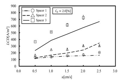
**Figure 7.** Limiting current density (numerical simulation and experiment [15]). The LCD obtained by our simulation reproduces the experimental results for Spacers 1 and 2. A comparison between LCD and the minimum effective Sherwood number shows correlations between them.
