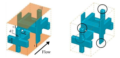
**Figure 8.** Spacer 4 structure, which has the geometric characteristics of  $\varepsilon = 0.81$ ,  $A_y/A_{mem} = 0.97$  and  $A_x = 11.78$  [mm<sup>2</sup>]. The spacer was devised based on our proposed design guidelines.
