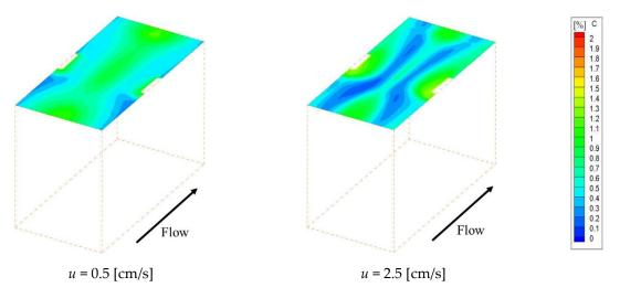
**Figure 10.** Concentration distribution when using Spacer 4. The spacer 4 can solve the problem that the low concentration region is formed due to the flow stagnation behind the structure.
