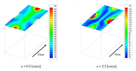
**Figure 11.** Effective Sherwood number distribution when using Spacer 4. The effective Sherwood number distribution is correlated with the concentration distribution on the membrane. The effective Sherwood number is high at places where the flow is disturbed around the structure, and the overall value is higher than that of the other spacers.
