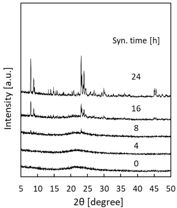
**Figure S2.** XRD patterns of obtained products prepared by gel-free SAC method for different synthesis times using unseeded uncoated silica support.
