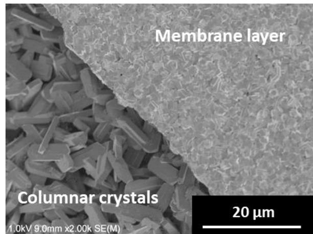
**Figure S1.** SEM image of silicalite-1 membrane fabricated by gel-free SAC method using uncoated silica support.
