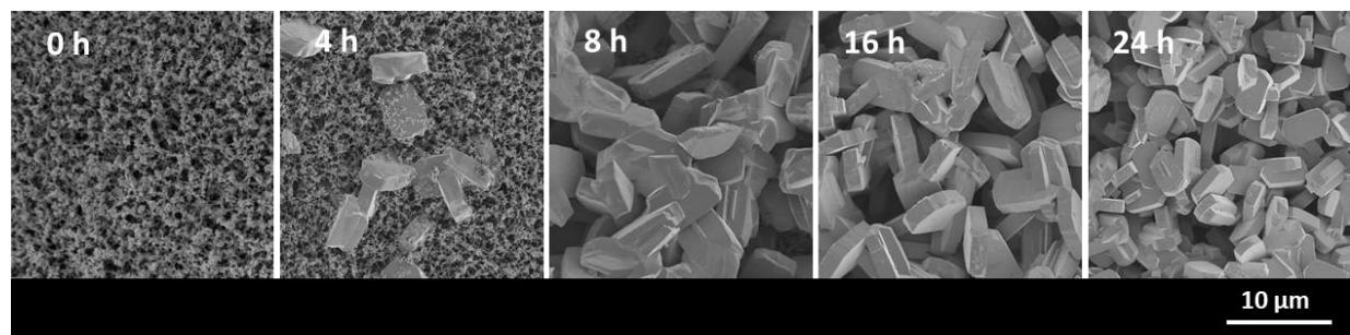
**Figure S3.** SEM images of obtained products prepared by gel-free SAC method for different synthesis times using unseeded uncoated silica support.
