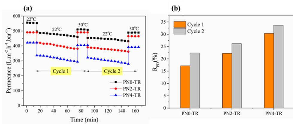
**Figure 7.** Protein fouling studies for biocatalytic membranes with and without PNIPAAm. (a) Permeance values for two filtration cycles; (b)  $R_{PD}$  after each filtration cycle (Error bars are in the range 1.1–2.9°). Experimental Conditions: Pressure = 100 kPa, cross-flow velocity = 12.6 cm/s, feed solution = 1 g/L BSA, 1 mM CaCl<sub>2</sub>, 7 mM NaCl, filtration temperature = 22 °C, cleaning temperature = 50 °C.
