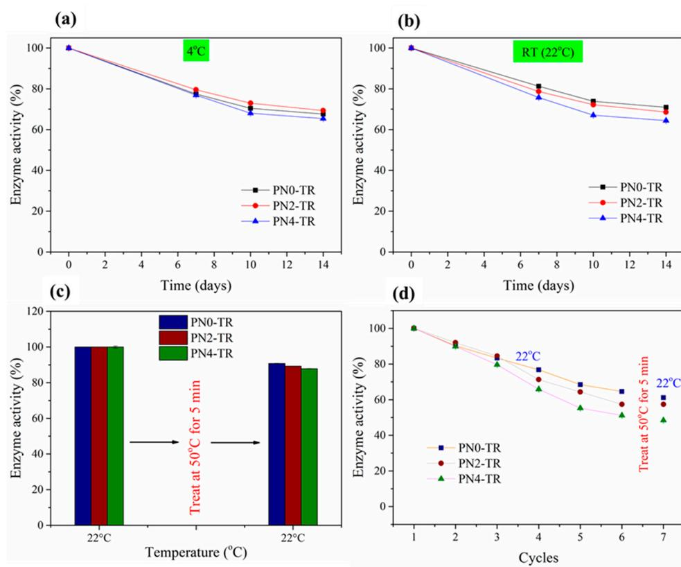
**Figure 8.** Hydrolytic activities of biocatalytic membranes for up to 14 days of storage at (a) 4 °C and (b) 22 °C; Stability of enzymes immobilized on to membranes in terms of enzyme activity with 50 °C treatment for 5 min after (c) one reuse cycle and (d) six reuse cycles.
