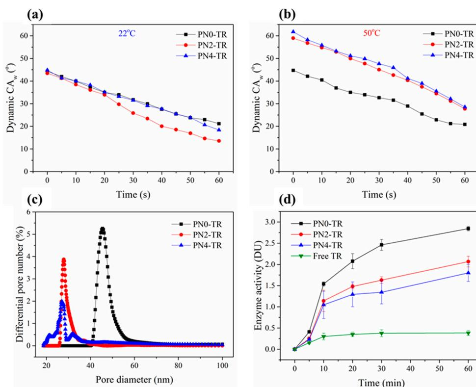
**Figure 4.** Dynamic water contact angles (CA<sub>w</sub>) of the biocatalytic membranes with and without PNIPAAm for 60 s contact time at (a) 22 °C (Error bars are in the range 0.56–0.89°); (b) 50 °C (Error bars are in the range 0.45–1.2°); (c) differential pore number (in %) distributions (Error bars are in the range 0.2–0.6%); (d) enzymatic activities of biocatalytic membranes over time with no PNIPAAm, 2 and 4 wt % PNIPAAm.
