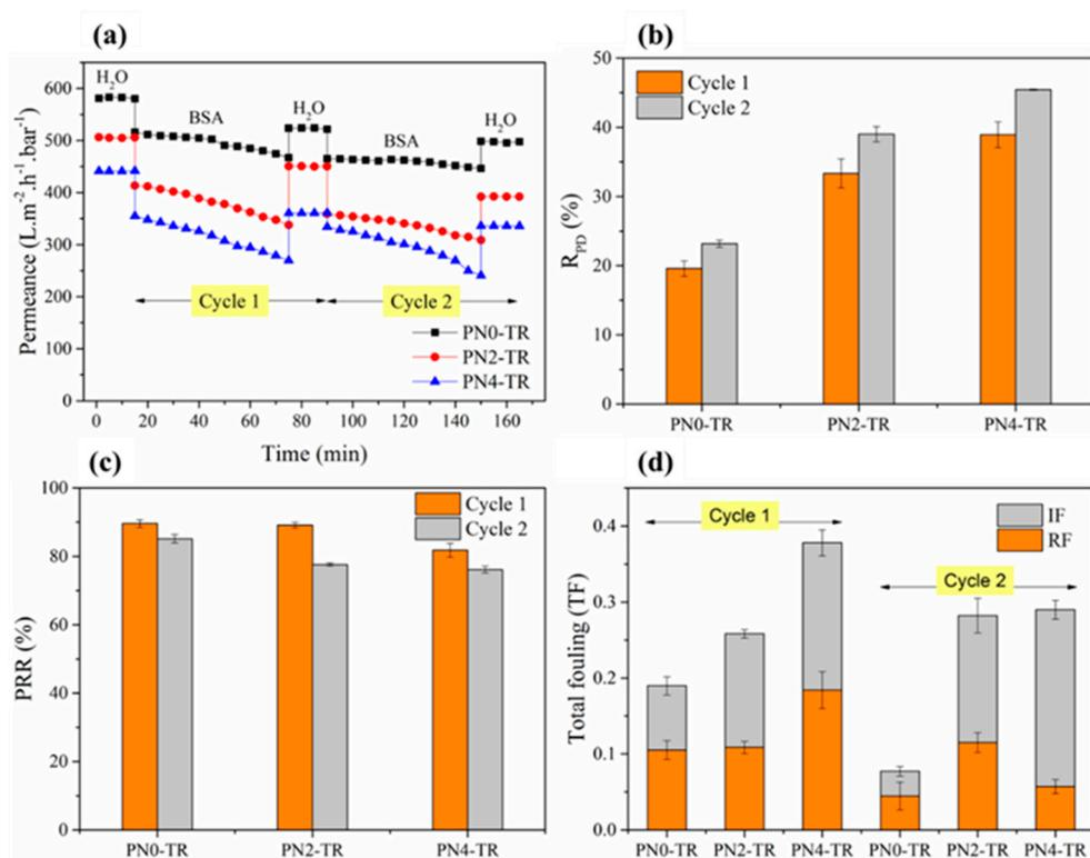
**Figure 5.** Protein fouling studies for biocatalytic membranes with and without PNIPAAm. (a) Permeance values for two filtration cycles; (b) R<sub>PD</sub> after each filtration cycle; (c) PRR after each filtration cycle; (d) RF, IF and TF for 2 filtration cycles. Experimental Conditions: Pressure = 100 kPa, cross-flow velocity = 12.6 cm/s, feed solution = 1 g/L BSA, 1 mM CaCl<sub>2</sub>, 7 mM NaCl, both filtration and cleaning temperature = 22 °C.
