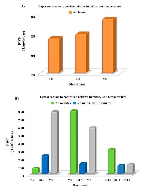
**Figure 4.** PWP of the membranes prepared via: (**A**) NIPS; (**B**) VIPS-NIPS (in all cases, the relative standard error was less than 5%).
