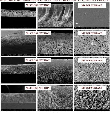
CASTING SOLUTION COMPOSITION: 15wt% PVDF, 5wt% PVP, 10 wt% PEG, 70wt% TEP
