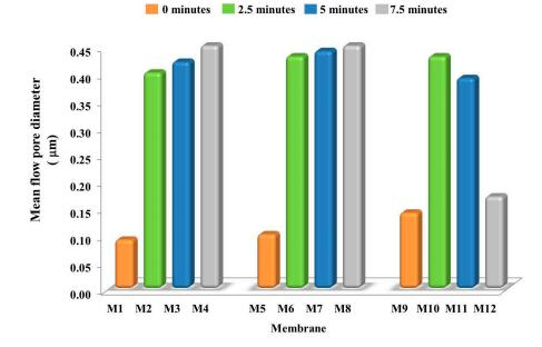
**Figure 3.** Mean flow pore diameter of the prepared membranes (in all cases, the relative standard error was less than 5%).
