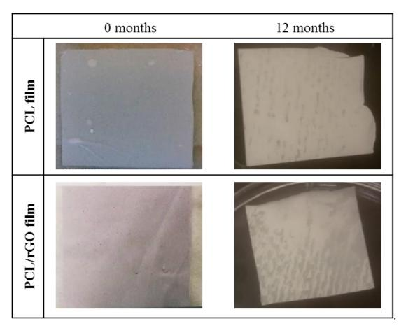
**Figure S3.** Photographs showing the visual aspect of the wet PCL and PCL/rGO membranes at 0 and 12 months of degradation (membrane pieces sizing 4×4 cm<sup>2</sup>).
