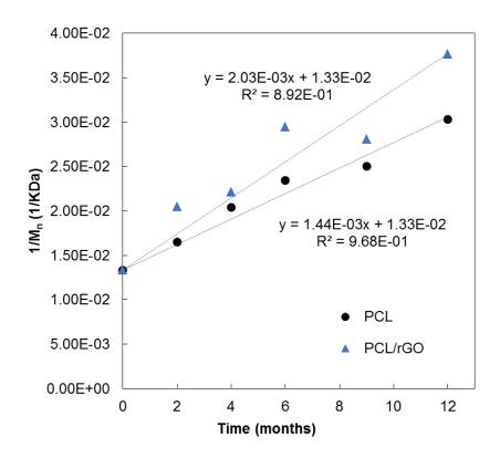
**Figure S1.** Kinetics of the hydrolysis of PCL and PCL/rGO membranes. Fitting of the molecular weight to the 2nd order hydrolysis kinetics (Equation S2) is depicted (dotted lines). For the present system  $M_0$  and  $C_w$  are the same for the PCL plain membranes and the PCL/rGO material as well as Mn0. Therefore from Figure S1, it can be extracted that k(PCL)/k(PCL/rGO) =  $(2.03 \times 10^{-3})/(1.44 \times 10^{-3}) \approx 1.4$ .
