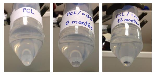
**Figure S2.** Photographs showing the rGO content at 0 and 12 months of degradation of the PCL/rGO membranes. (PCL is shown as control).
