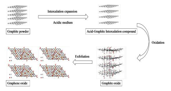
Figure 3. Schematic illustration of GO preparation process.
