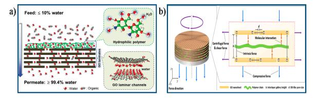
**Figure 9.** Schematic diagram of the process for improving separation performance of GO membranes: (a) Schematic illustration of the integrated GO membrane combined an ultrathin surface water-capturing polymeric layer with GO layers [116]. Copyright 2015 John Wiley and Sons; (b) Schematic illustration of the process to tune 2D channels of GO membrane with external force [55]. Copyright 2016 American Chemistry Society.
