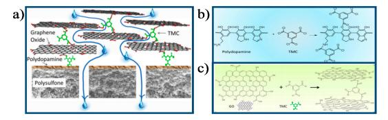
**Figure 10.** Schematic illustration of (**a**) The forming process of the GO membrane; (**b**) The interaction mechanism between PDA and TMC; (**c**) The interaction mechanism between GO and TMC [26]. Copyright 2013 American Chemistry Society.
