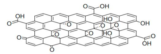
Figure 1. Structure mode of graphene oxide [23]. Copyright 2015 Journal of the Physical Society of Japan.
