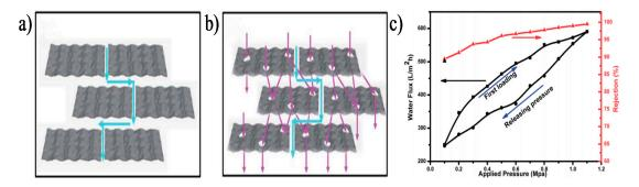
**Figure 8.** Schematic diagrams of transport path of (**a**) Original GO; (**b**) Mesoporous GO membrane; (**c**) The separation property of mesoporous GO membrane [114]. Copyright 2014 Royal Society of Chemistry.
