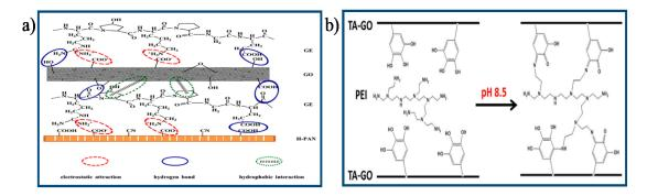
**Figure 11.** (a) Schematic illustration of the interfacial interaction in GO-based hybrid membrane [121] Copyright 2015 Elsevier; (b) Schematic illustration of the formation of covalent bonding between adjacent TA–GO sheets [124]. Copyright 2016 Elsevier.
