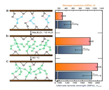
**Figure 12.** Left: Schematic diagram of the formation of covalent bonding between GO sheets and borate ion. (**a**) Water molecules bound the GO sheets through hydrogen bond; (**b**) Borate anions bound to the GO sheets through covalent bond; (**c**) More covalent bonds formed within the GO sheets after thermal annealing. Right: Mechanical strength of respective films [49]. Copyright 2011 John Wiely and Sons.
