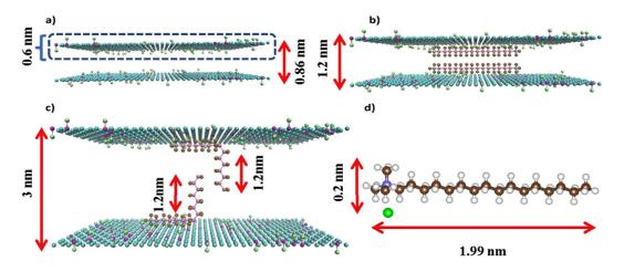
**Figure 6.** Schematic illustration of possible arrangement of C16TAB within GO membranes: (**a**) The pure GO membrane; (**b**) Two C16TAB paralleled to GO plane; (**c**) Two C16TAB perpendicularly arranged to GO laminate plane; (**d**) Molecular structure of C16TAB with C1–N chain length about 1.99 nm [96]. Copyright 2017 Elsevier.
