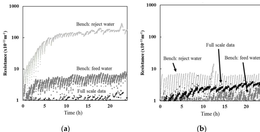
**Figure 2.** Results from filtration tests: (a) Barrie Surface WTP; and (b) Lakeview WTP. Full-scale resistance data are plotted for comparison.
