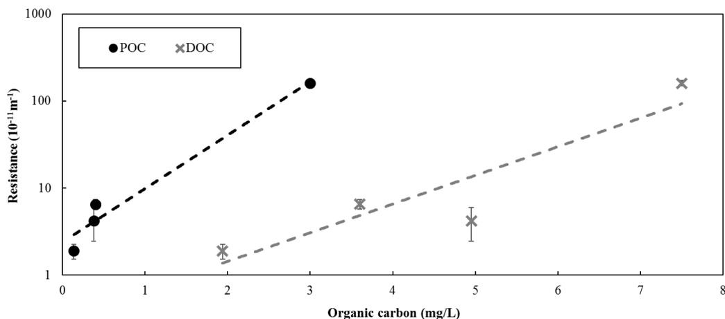
**Figure 3.** Resistance (averaged over the entire last permeation cycle) for each of the bench-scale filtration tests vs. organic carbon concentration (POC, DOC) in the solution filtered. The error bars represent the standard error associated with the resistance of the last permeation cycle. Exponential relationship was fitted to the data presented to illustrate the overall trend.
