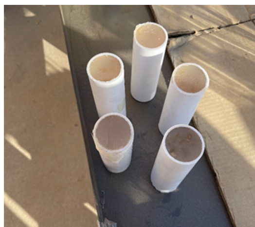
Figure 2. Preparation of the agarose–KCl–NaCl salt-bridge separator before installation between the anode and cathode chambers.
