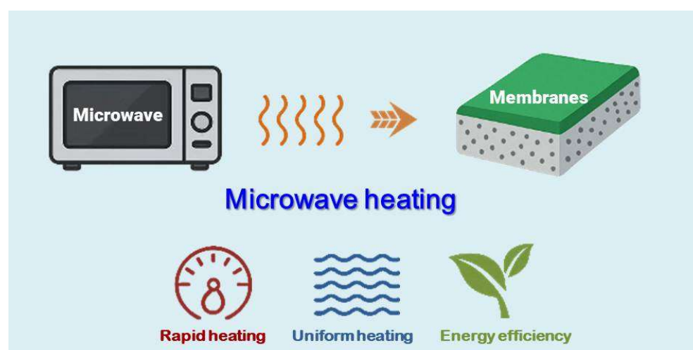
Figure 1. Membrane fabrication on a substrate via microwave synthesis.
