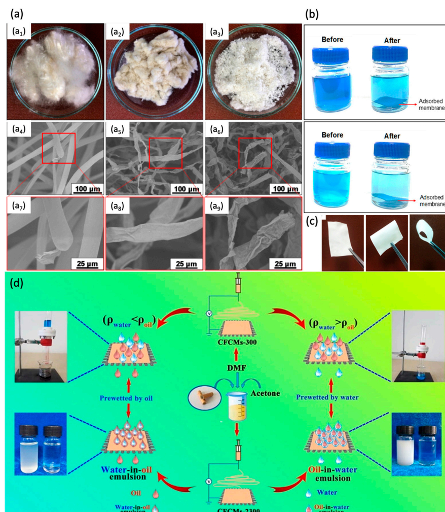
Figure 10. Membranes fabricated via cellulose and their derivatives: (a) morphology of kapok fiber derived membrane ((a 1 –a 3 ) refers to raw kapok fiber, cellulose microfiber after NaOH treatment, and cellulose microfiber after NaClO 2 treatment, respectively. While (a 4 –a 9 ) refer to their SEM morphologies at different resolutions); (b) digital photo of methylene blue before and after adsorption; (c) digital photos of the fabricated membrane showing [135]; (d) schematic illustration of CA (derived from cigarette) membrane fabrication and its performance evaluation [138]. Reprinted with copyright permission.
