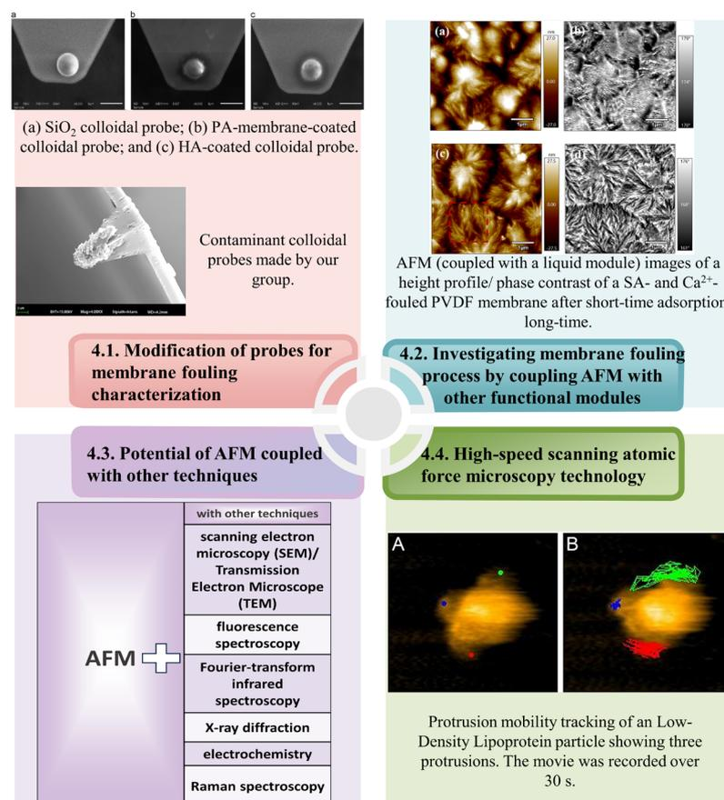
**Figure 9.** Application of improved AFM technology membrane fouling research, where the AFM images are reproduced from [55,72,95], with permission from Elsevier academic publishing company.
