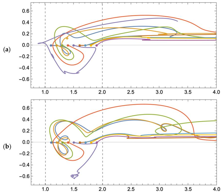
**Figure 10.** Trajectories of particles uniformly spaced along the boundary of the membrane surface cavity and feed channel, subject to a rapidly pulsed feed flow: (a) average  $Re = 600$ ; (b) average  $Re = 1600$ .
