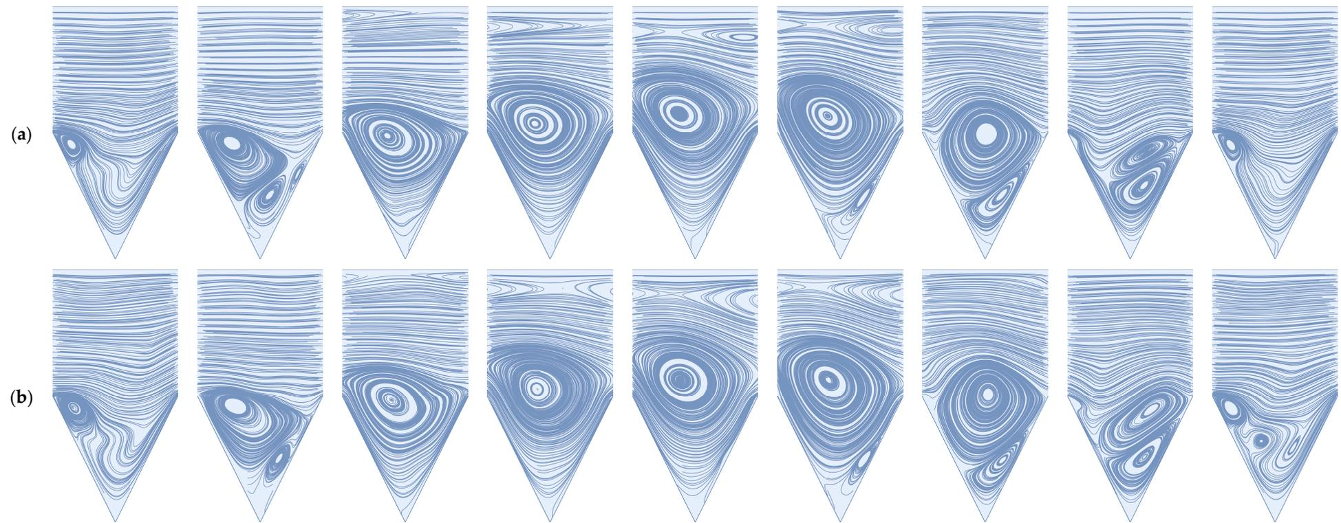
**Figure 5.** The deep sweep followed by a vortex ejection for a rapidly pulsed feed flow and a permeate flux condition of 1/2000 the maximum inlet flow velocity: (a) average flow  $Re = 600$ ; (b) average flow  $Re = 1600$ .
