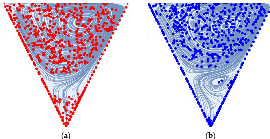
**Figure 9.** Final cavity particle positions for a steady feed flow condition (see Figure 8) are driven by the locations of the recirculation zones in the membrane surface pattern: (a)  $Re = 600$ ; (b)  $Re = 1600$ .
