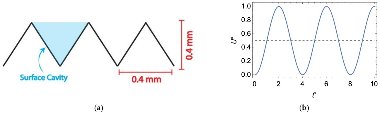
**Figure 2.** (a) Triangular membrane surface pattern studied in this work; (b) the sinusoidal waveform used to modulate the average inlet flow velocity,  $U$ , where  $*$  denotes a dimensionless variable—see Equation (7).
