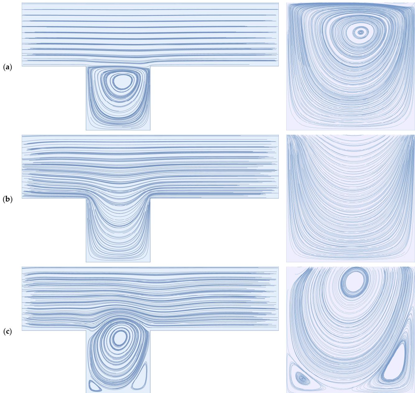
**Figure 1.** (a) A stationary cavity vortex driven by a steady feed flow with a Reynolds number of 100; (b) the deep sweep mechanism resulting from a sudden increase in flow volume; (c) the vortex ejection mechanism resulting from a sudden decrease in flow volume.
