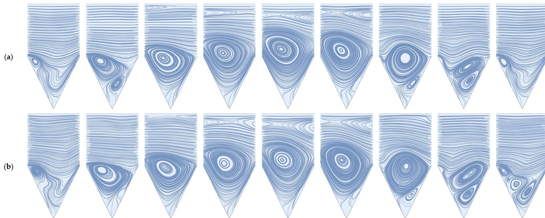
**Figure 6.** The deep sweep followed by a vortex ejection for a rapidly pulsed feed flow and an increased permeate flux condition of 1/200 the maximum inlet flow velocity; (a) average flow  $Re = 600$ ; (b) average flow  $Re = 1600$ .
