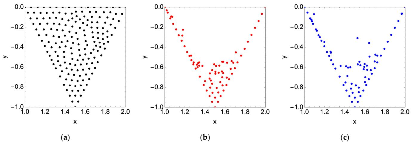
**Figure 11.** (a) Initial arbitrary cavity particle positions; (b) final cavity particle positions after 4 pulses of the feed flow with an average  $Re = 600$  (red); (c)  $Re = 1600$  (blue).
