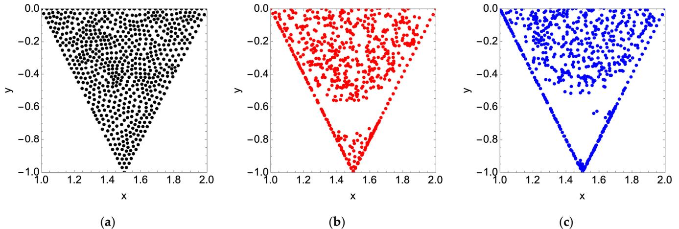
**Figure 8.** (a) Initial arbitrary cavity particle positions; (b) final cavity particle positions for a steady feed flow condition and dimensionless simulation time of 200 with  $Re = 600$  (red); (c)  $Re = 1600$  (blue).
