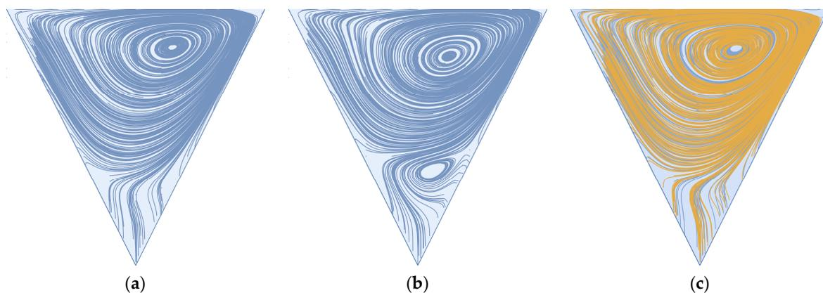
**Figure 4.** (a) Vortex formation in a single cavity exposed to steady flow for  $Re = 600$ ; (b)  $Re = 1600$ ; (c) comparison of stream plot lines in the first (blue) and last (yellow) cavities of sequential cavity geometry (see Figure 3).
