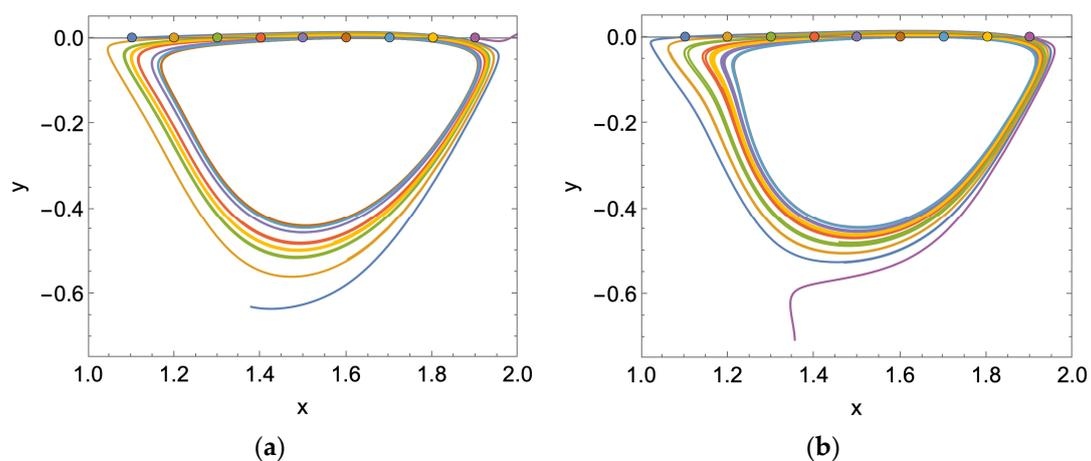
**Figure 7.** Trajectories of particles uniformly spaced along the boundary of the membrane surface cavity and feed channel, subject to a steady flow: (a)  $Re = 600$ ; (b)  $Re = 1600$ .
