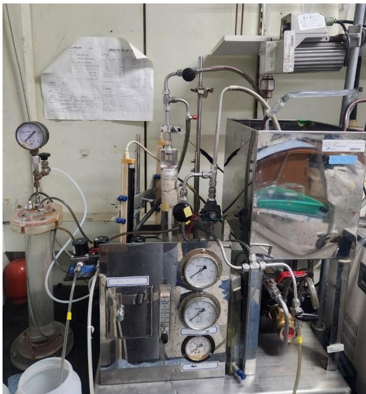
**Scheme 2.** The combined water treatment system of the tubular MF membrane and titanium dioxide-immobilized PES beads with intermittent water backwashing and UV radiation.
