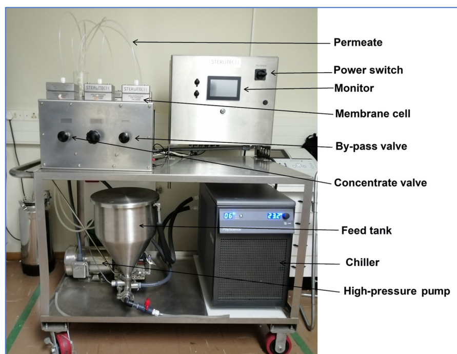
Figure 1. Crossflow filtration unit used for flux, rejection and fouling experiments.
