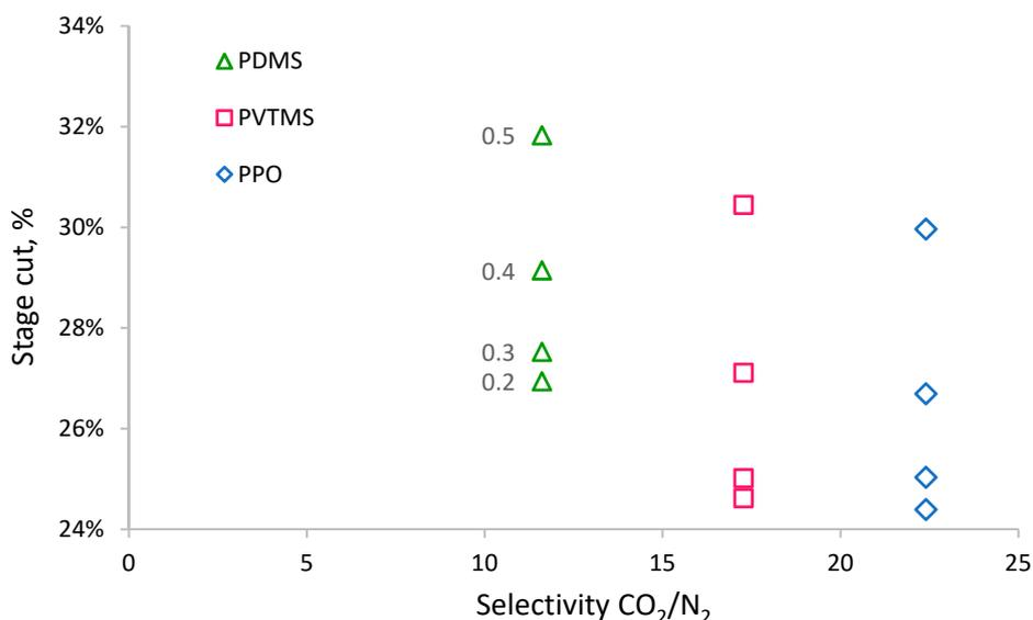
**Figure 6.** The dependence of stage cuts on the selectivity of CO<sub>2</sub>/N<sub>2</sub> for achieving 50% CO<sub>2</sub> recovery at different permeate pressures (numbers near markers).
