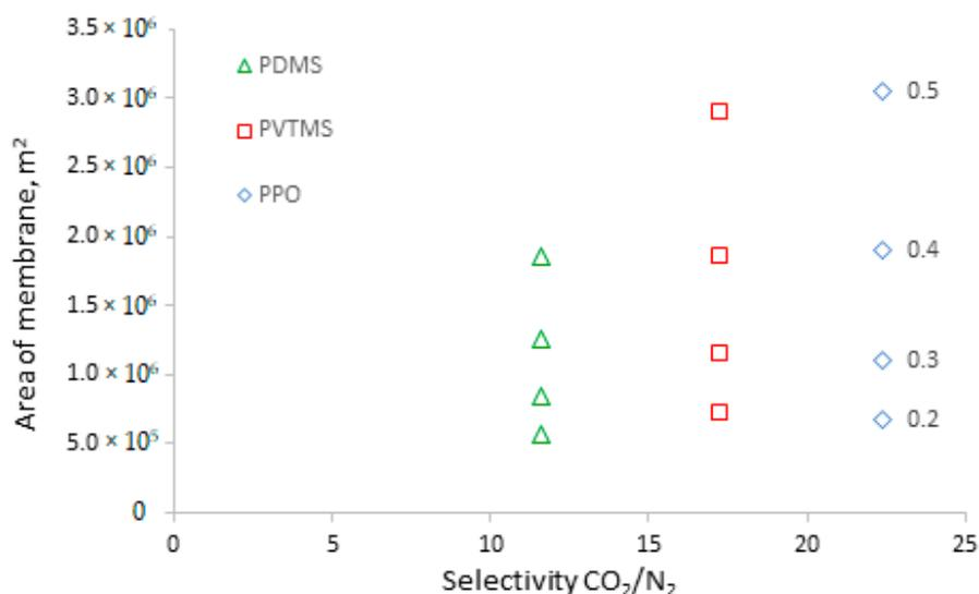
**Figure 5.** The dependence of membrane area on the selectivity of CO<sub>2</sub>/N<sub>2</sub> for achieving 50% CO<sub>2</sub> recovery at different permeate pressures (numbers near markers).
