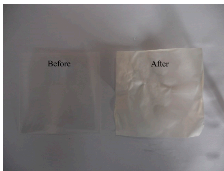
Figure 1. Macrographs of membrane material before (left) and after (right) adsorption.
