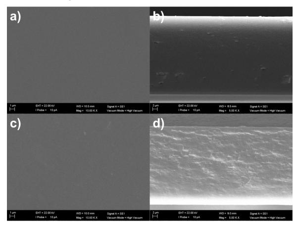
**Figure 3.** SEM surface and cross-section view images of the fabricated membranes based on CS and L-proline:xylitol DES. (**a**,**b**) crosslinked chitosan and (**c**,**d**) crosslinked chitosan:L-proline: xylitol (CS:PRO:XYL).
