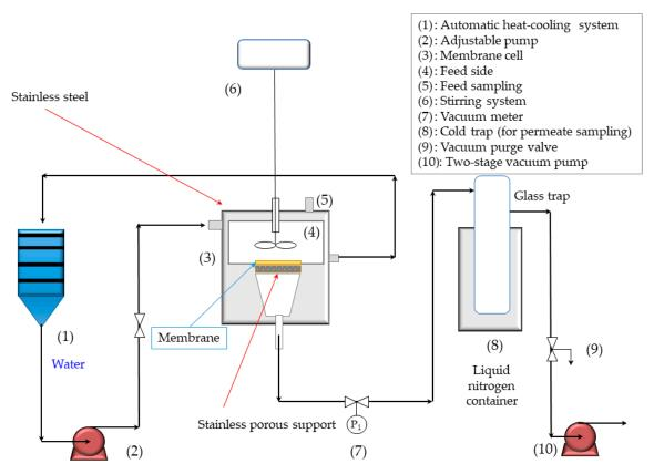
Figure 1. Graphical depiction of the experimental set-up used in PV experiments.
