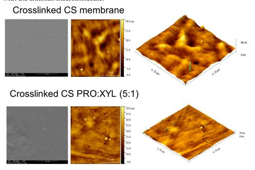
**Figure 4.** AFM surface and 3D images ( $15 \times 15 \mu m$ ) of pristine CS and CS:PRO:XYL membranes.
