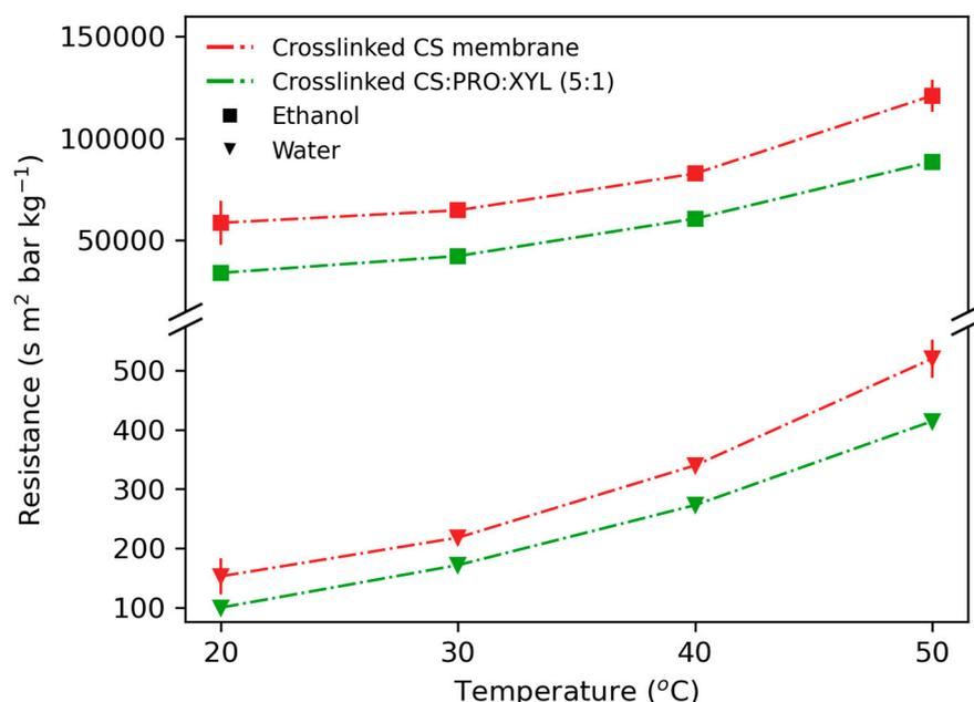
**Figure 9.** Comparison of ethanol and water mass-transfer resistance through membranes. Points connecting lines are to improve readability of the graph.
