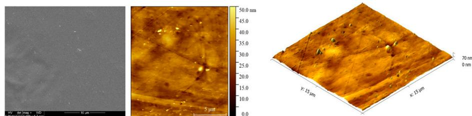
**Figure 4.** AFM surface and 3D images ( $15 \times 15 \mu\text{m}$ ) of pristine CS and CS:PRO:XYL membranes.
