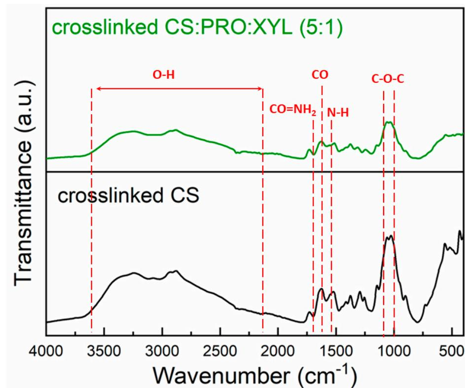
**Figure 2.** FTIR spectra for pristine crosslinked CS and CS:PRO:XYL membranes.
