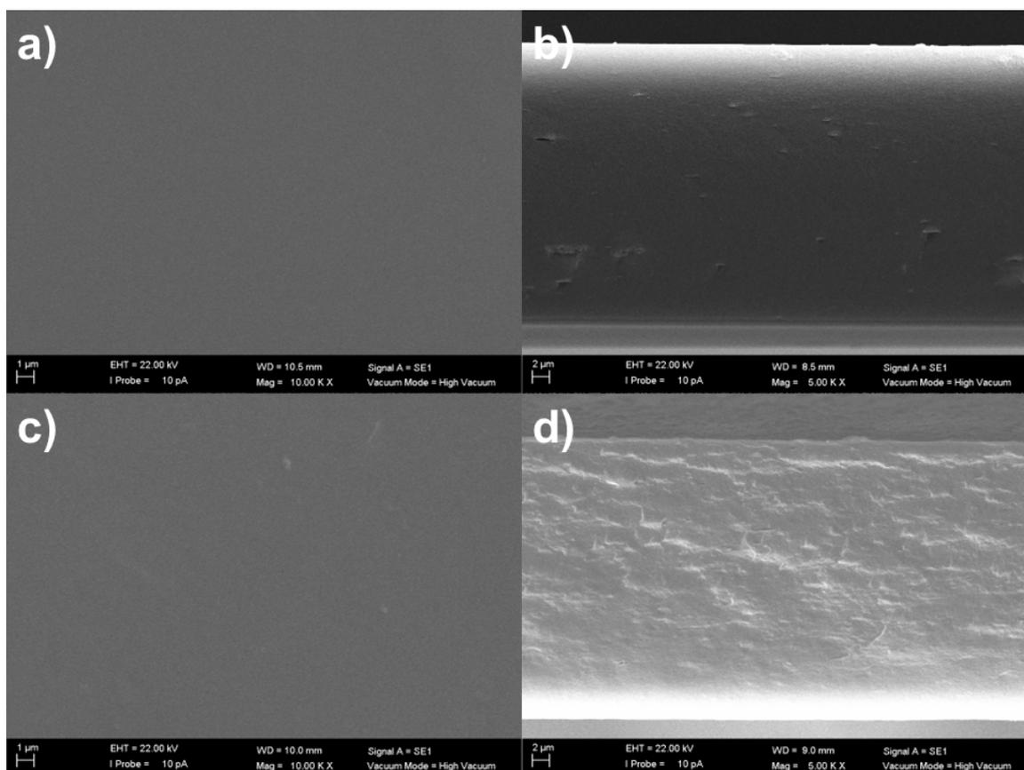
**Figure 3.** SEM surface and cross-section view images of the fabricated membranes based on CS and L-proline:xylitol DES. (a,b) crosslinked chitosan and (c,d) crosslinked chitosan:L-proline: xylitol (CS:PRO:XYL).
