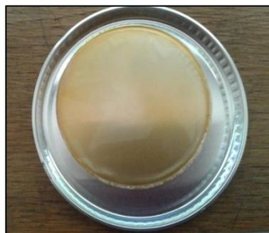
**Figure 9.** Polymer inclusion membrane (PIM) composed of 45% wt. CTA, 40% wt. di(2-ethylhexyl) phosphoric acid and 15% wt. acetylated lignin. Adapted from [91,92].
