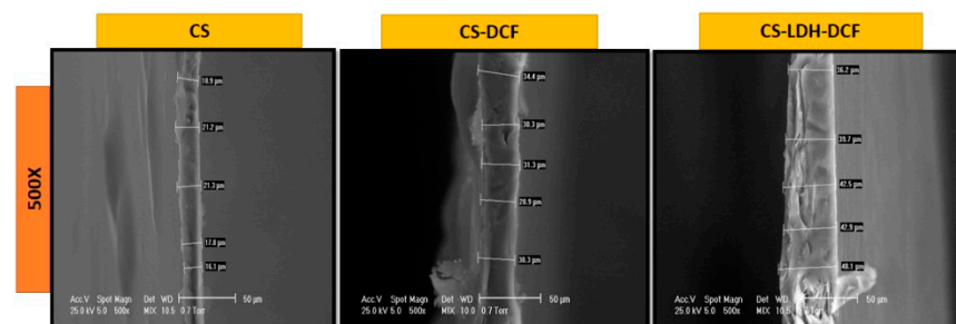
Figure 3. SEM images of the cross-section view of chitosan, chitosan loaded with diclofenac, and chitosan-LDH loaded with diclofenac.
