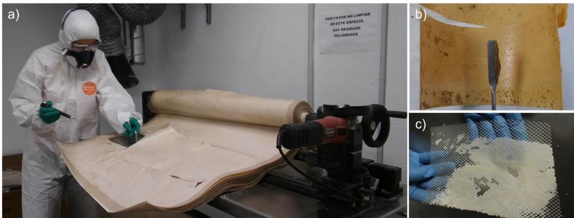
**Figure 4.** (a) Opened RO module and extraction of membrane and spacer samples. Reproduced with permission from Ref. [105]. Copyright 2022, A. Lejarazu-Larrañaga et al., (b) taking membrane fouling samples for analysis (presumably organic fouling), (c) a sample of a turbulence promoter (feed spacer) with scaling deposits.
