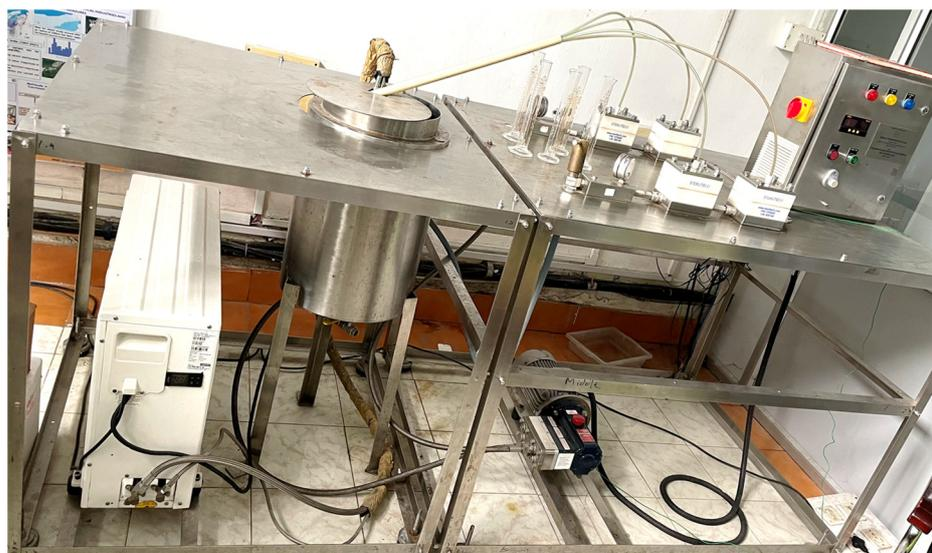
**Figure 2.** The crossflow NF/RO (Nanofiltration/Reverse Osmosis) four-cell membrane testing unit.
